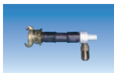
Art. No. 1700018300 Vacuum adapter for rapid deflation of the support frame. Connection of snap-coupling to the air source, pressure should be between 4 and 6 bar (58 and 87 psi)
